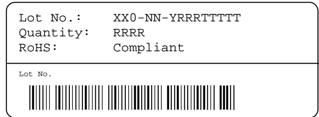
Figure 14: First label on reel: XX = Sensor Type (71 for SHT71), NN = Chip Version (04 for V4), Y = last digit of year, RRR = number of sensors on reel divided by 10 (200 for 2000 units), TTTTT = Traceability Code.
